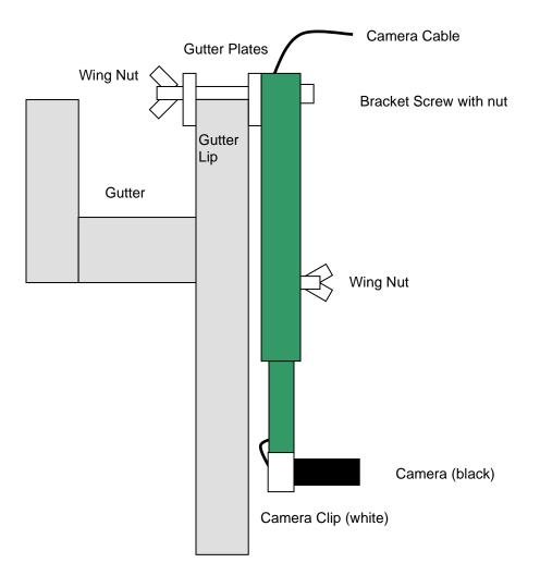
After the wing nut is tight, check that the bracket screw is parallel to the top of the gutter lip and that the shaft is parallel to the wall.
